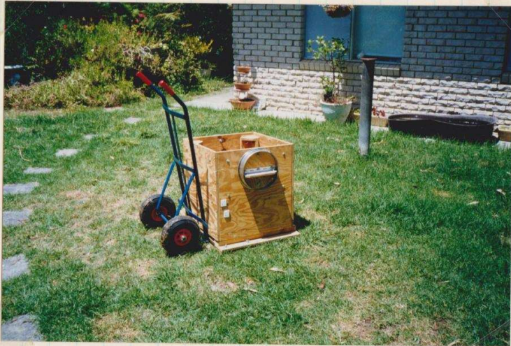
TWO TEFLON "SPACER BEARINGS" TO LEFT OF MIRROR BOX ENHANCE RIGIDITY OF ROCKER BOX MIRROR BOX UNIT AND LOWER CENTRE OF GRAVITY AND THRUST WHEN TURNING IN AZIMUTH LATERAL THRUST BEARINGS
