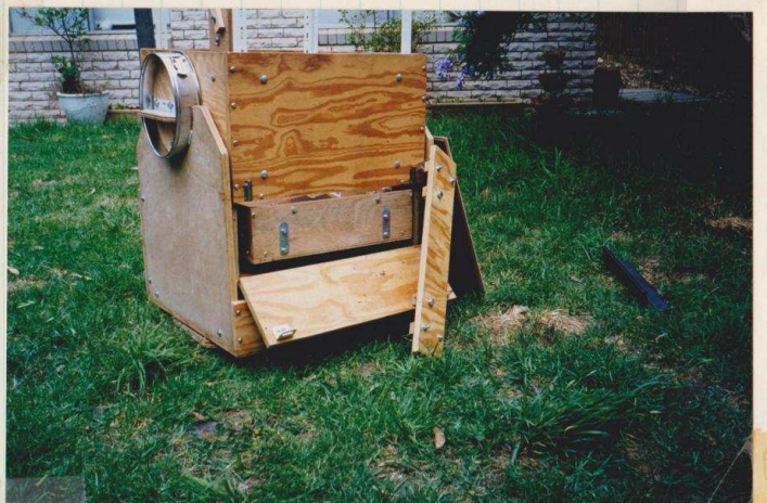
MIRROR BOX IN ROCKER BOX, HATCH OPEN WITH MIRROR CELL PARTLY INSERTED SITTING ON 20 INCH PLATE OF 1/2 INCH STEEL. MIRROR CELL POSITIONING BAR / GUIDE ON RIGHT
